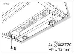
Secure the appliance to the brackets using two screws on each side.
